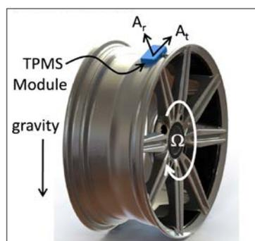
Tire pressure monitoring system (TPMS) module mounted to a rim.
