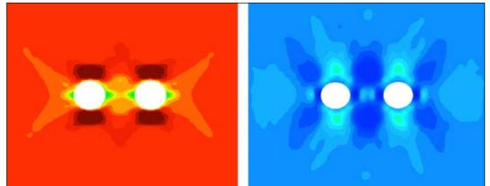
Artificial linear superposition result of two pores from the single-pore simulation results: (left) axial stress and (right) transverse stress.
