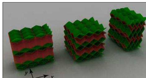
Cellular structure actuated by differentially pressurizing two sets of tubes in  $x$  and  $y$  directions.
