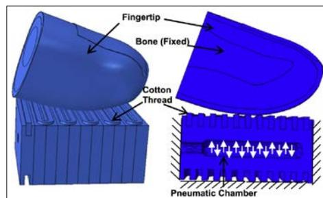
3D modeling of the inflation behavior of the silicone pneumatic chamber with a fingertip contacting the top surface: (left) integral structure, (right) cross section.
