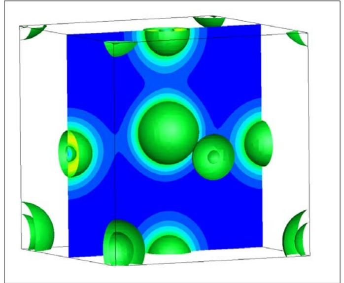
Plot of the electron density within a unit cell of lead titanate at the lowest energy tetragonal state. Titanium is the center atom and lead is on each corner.
