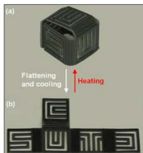
A directly printed origami SUTD-CU box. An as-printed 3D SUTD-CU box in (a) was deformed into a flat form at  $T_L$  in (b). After heating back to  $T_H$ , the structure recovers the 3D box shape.
