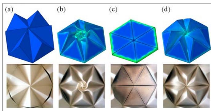
Maximum principal strains in the hexagonal cell from FE analysis and the geometries of the manufactured demonstrator; (a) deployed state, (b) transition from deployed to retracted state, (c) retracted state, (d) transition from retracted to deployed state.
